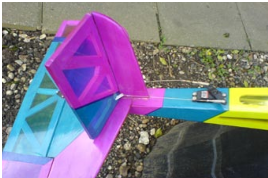
Figure 8. The rudder pull-pull control system
