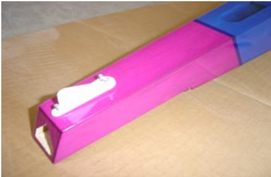
Figure 3. Install the tail skid
