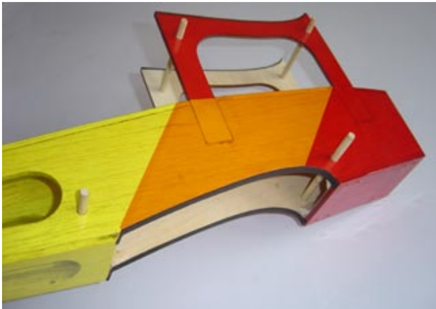
Figure 13. Glue wood dowels and stick rubber strips
