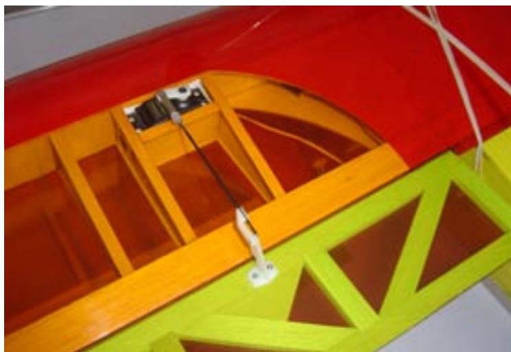
Figure 12. Install aileron servos and connect push-rods
