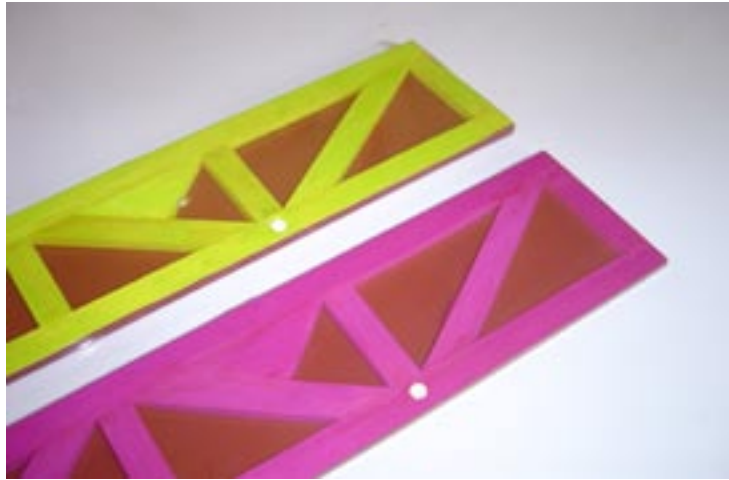
Figure 11. Glue ball cups in the holes on the ailerons
